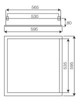
All dimenions are in mm. Tolerance + 2 mm.
