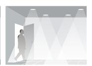
Light level automatically adjusts to maintain required lux levels by detecting available daylight
