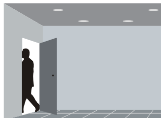
Lights turn off if no presence detected
