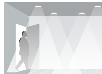
Lights turn on if presence detected
