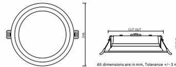
All dimensions are in mm, Tolerance +/- 3 mm
