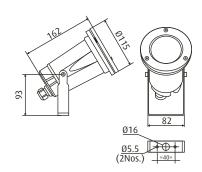
All dimensions are in mm. Tolerance ± 2 mm
